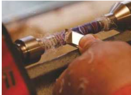
▲ Pic.8 A final pass with a skew can be made to get things as clean as possible
